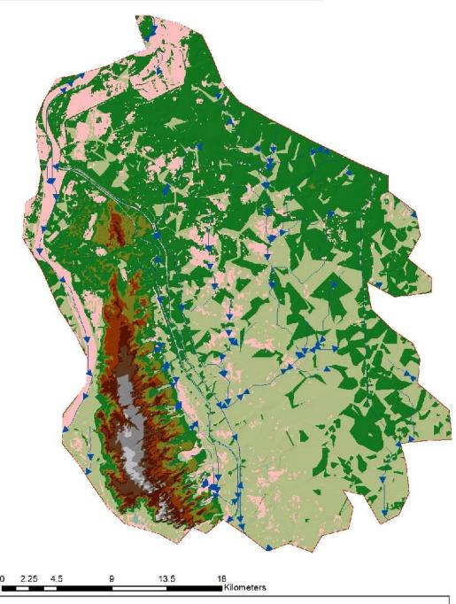
5 m Digital Elevation Model (DEM) has been used to generate surface topography of the district. The same product was used to extract natural drainage / gradients / flow directions. This map can be useful for determining route(s) for safe dewatering of flood water
